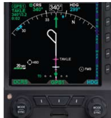
Figure 2-36 ARC CDI Mode with Base Map
