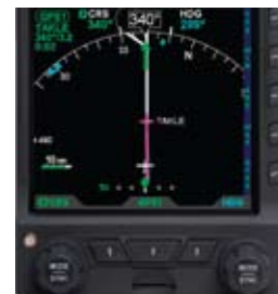
Figure 4-35 ARC CDI Compass Mode
