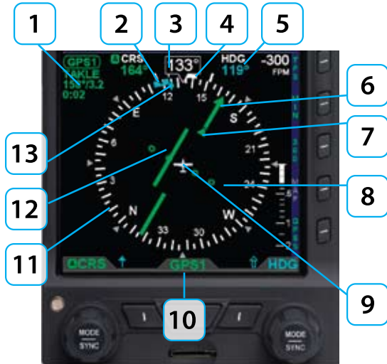
Figure 4-32 Horizontal Situation Indicator
