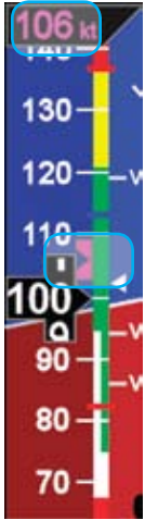
Figure 4-7 Airspeed Bug Selected to Edit
