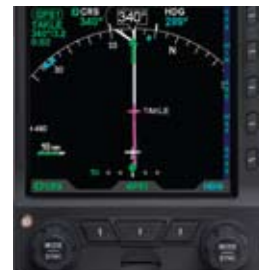
Figure 3-30 ARC CDI Compass Mode
