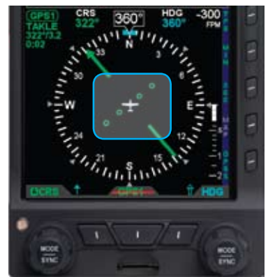
Figure 4-58 No Course Deviation Bar or FROM/TO Info
