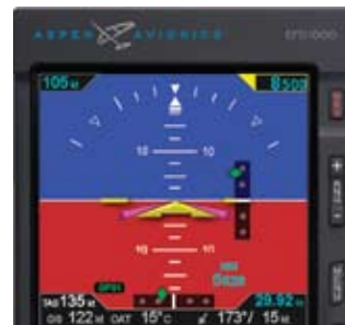
Figure 4-29 Altitude Tape Disabled
