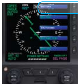
Figure 6-6 Menu, POWER SETTINGS, Page 6 of 7, Key 1
