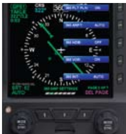
Figure 5-8 360° Compass Mode Display Options
