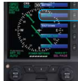
Figure 6-7 Menu, POWER SETTINGS, Page 6 of 7, EXT PWR Menu Key (Key 2)
