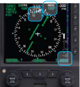
Figure 3-10 Heading Field Disabled
