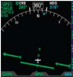
Figure 4-42 Reduced Length Course Pointer
