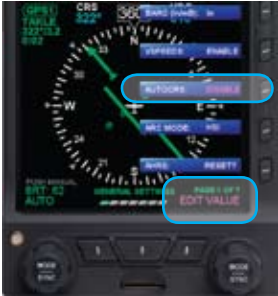
Figure 2-23 EDIT VALUE Displays Above Right Knob
