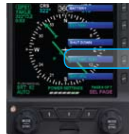
Figure 6-8 Menu, POWER SETTINGS, Page 6 of 7, EXT PWR Menu Key (Key 4)
