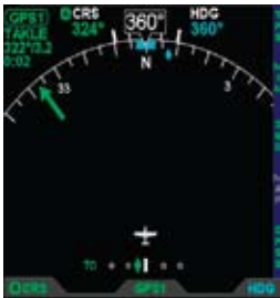
Figure 4-43 Stub Course Arrowhead
