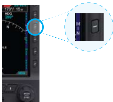
Figure 3-32 MIN Hot Key (shown disabled)
