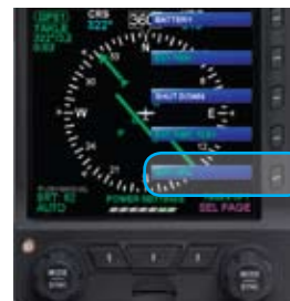
Figure 6-9 Menu, POWER SETTINGS, Page 6 of 7, BAT Menu Key (Key 5)
