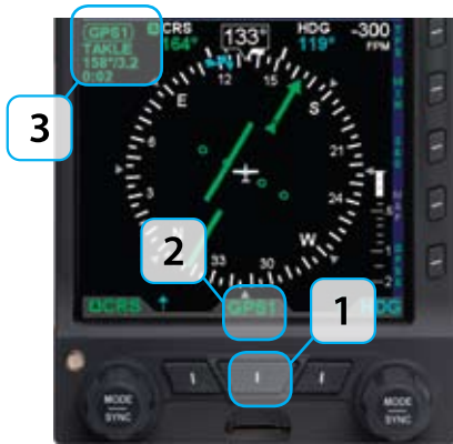
Figure 4-56 Navigation Source Information Block
