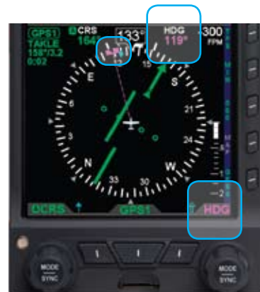
Figure 4-77 Heading Selected to Edit
