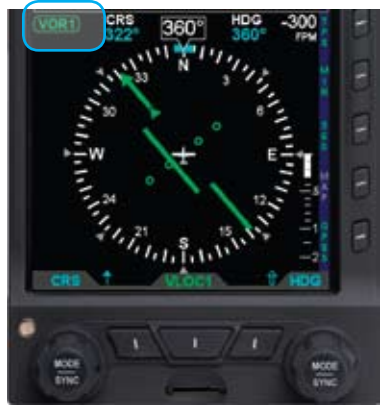
Figure 4-60 Blank Info Block Fields
