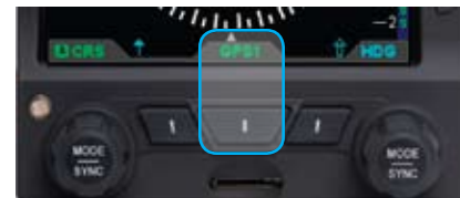
Figure 3-11 CDI Navigation Source Selection Button
