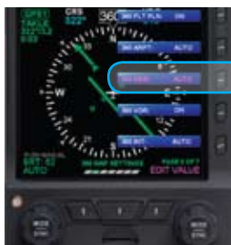
Figure 5-11 360° NDB Display Option Set To OFF
