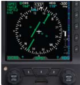
Figure 4-70 NO bearing pointers or source information
