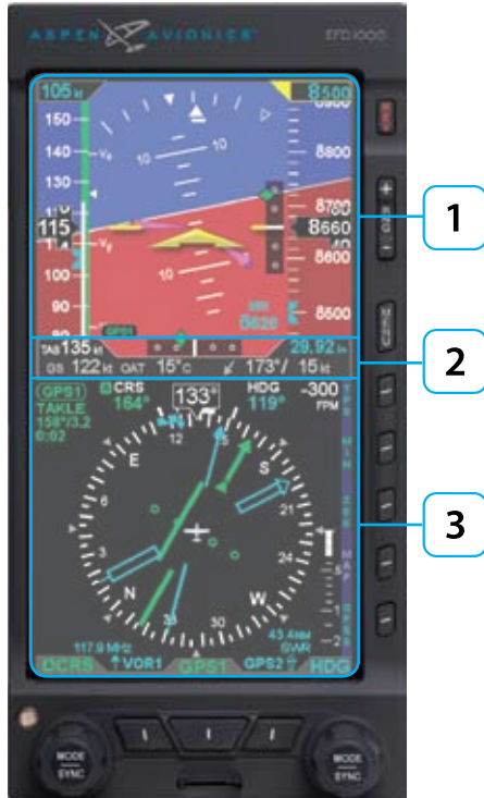
Figure 2-26 EFD1000 Pro PFD Display Areas
