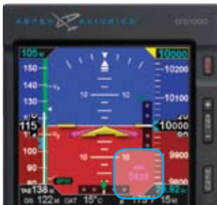
Figure 3-33 MIN Display Selected for Editing
