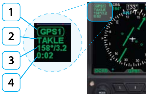
Figure 4-57 CDI Navigation Source Information Block
