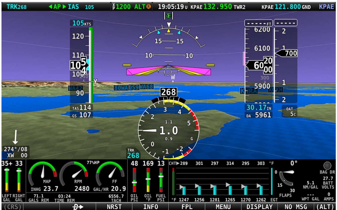
Figure 3: Example of G Meter Being Displayed
